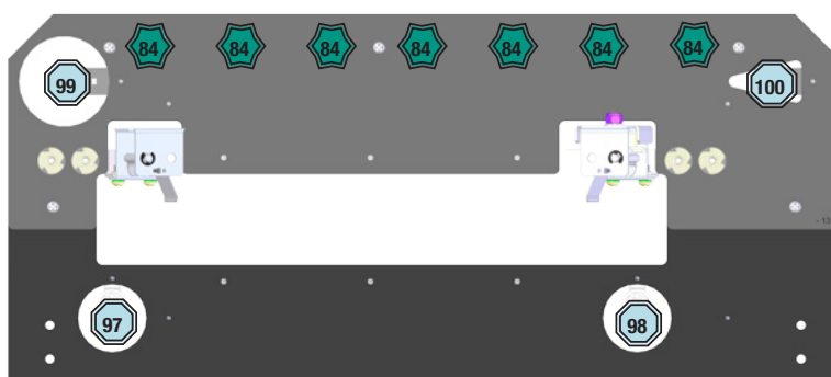
Figure 3.2.5. Playfield back panel lighting locations.
